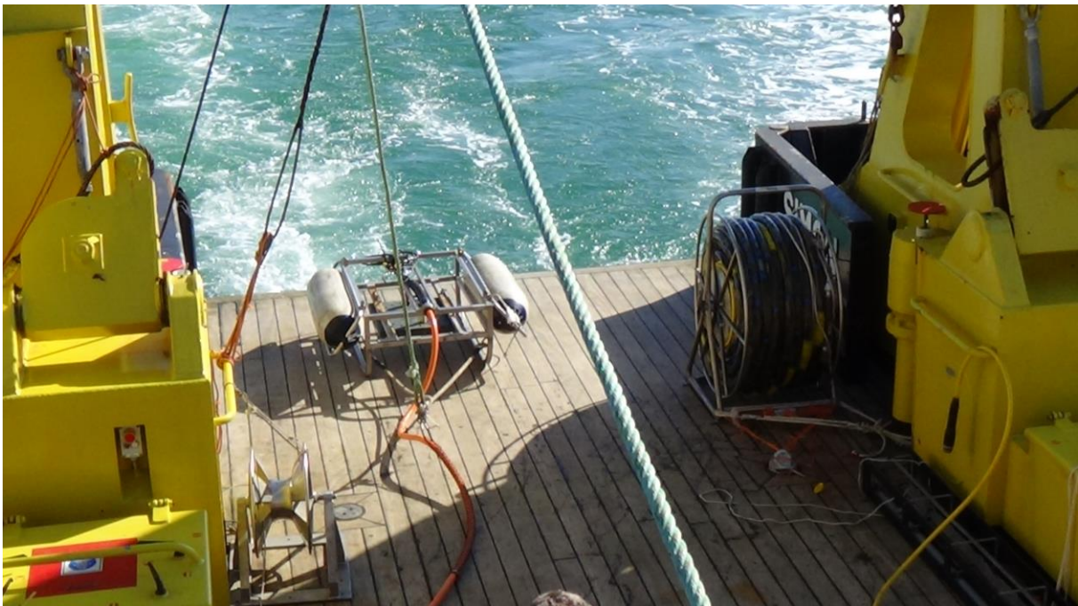
Figure 2: HF boomer of Deltares attached to the A-frame of the ship.
