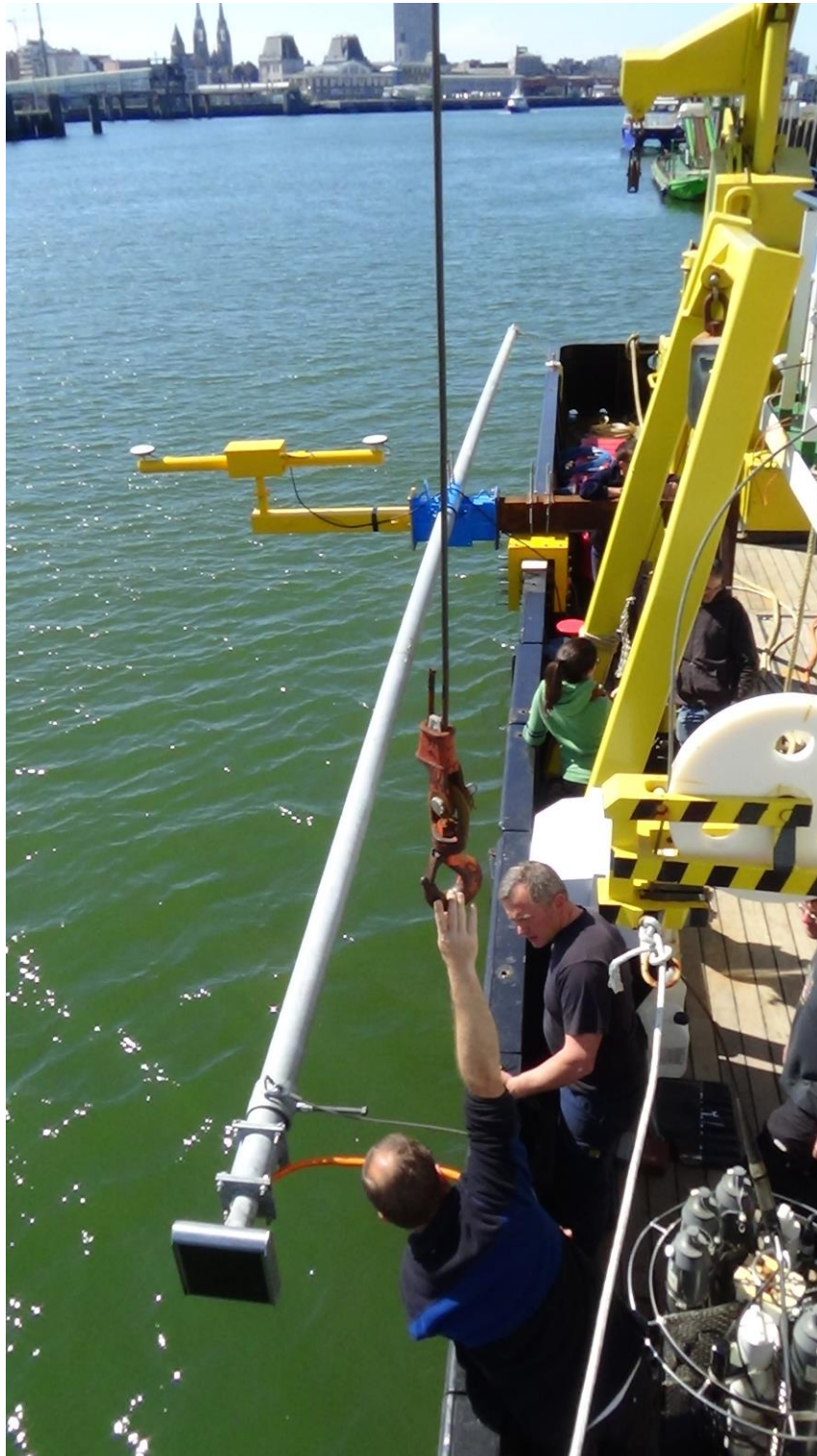
Figure 3: Fixed mounting for the PES and Geopulse. Here the PES is attached to the mounting pole.
